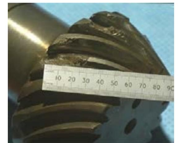
*Damaged teeth of a transmission cog*
